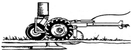
The burrow builder mechanically delivers poisoned bait underground to economically control pocket gophers on large acreages. A tractor pulls the burrow builder. The device consists of a knife and torpedo assembly that makes an artificial burrow at desired soil depths.
